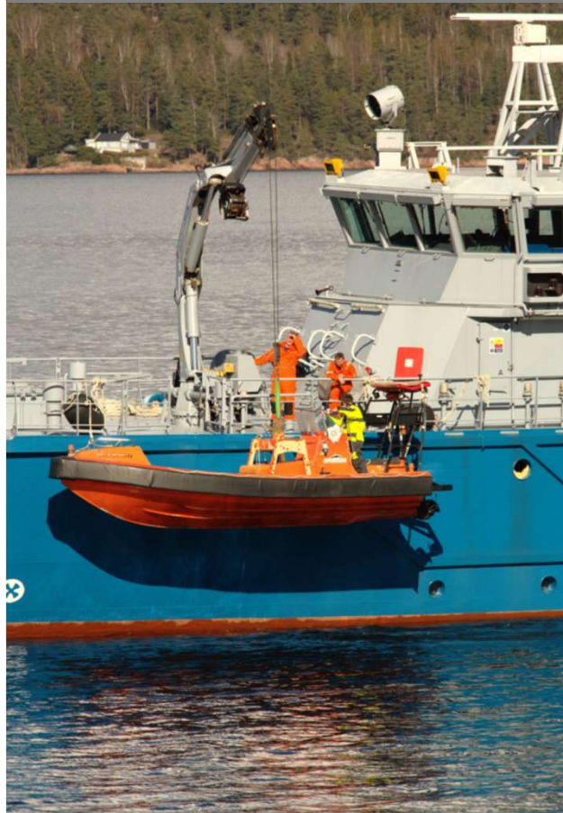
8 meter Springer self righting FRC on the foredeck. Speed max 32 knots. Capacity 15 persons
