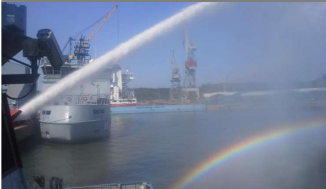
Remote controlled FiFi monitor with foam capacity.
