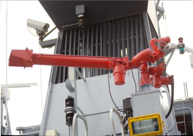
Remote controlled FiFi monitor with foam capacity.
