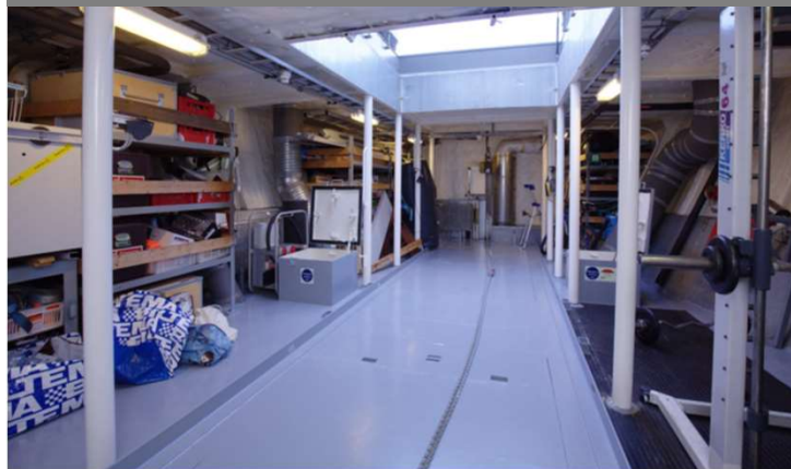
136 m3 cargo hold under the fore deck with cargo hatch and deck crane access
