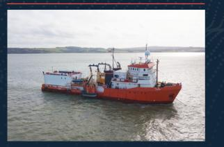
Versatile. rugged former North Sea SBSV (Standby Safety Vessel) converted to a Vessel Borne Armoury with enhanced accommodation and welfare facilities.
